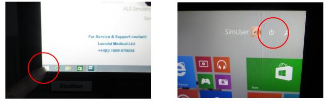
3. Turn off Instructor PC in control room by clicking End Session button on tool bar. Choose "Discard Result and EXIT" then "Exit LLEAP only". Shutdown ALL programmes open on the tool bar before shutting down PC by right clicking on icons and selecting close window. Select Windows icon on bottom left hand side of screen, press power options and select Shut Down.
