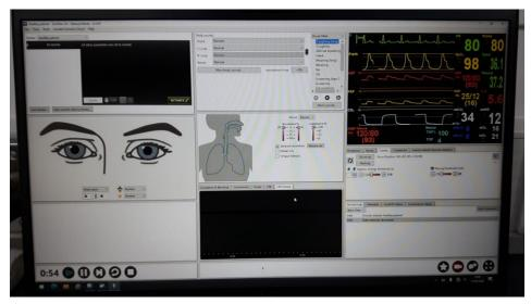
8. SimMan 3G Plus has a USB headset and microphone connected to the Instructor PC, to speak through the manikin activate the microphone by clicking the speech bubbles icon on bottom right of screen. Mic can be muted by clicking mute button on headset cable.
