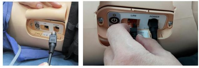
5. Open floor panel and plug in SimMan's power cable and LAN cable to relevant sockets, switch on power.
